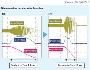
2.3 sec. reduction of deceleration time without a braking resistor is achieved when the function is active.
