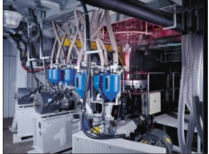
Baldor vector drive on a blown film extruder.
